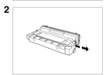
Remove the protective seal.
